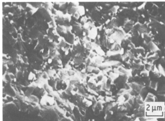
Figure 2 SE micrograph of a fracture surface of AlN hot-pressed at 27 MPa, 1700^\circ C for 1 h.
